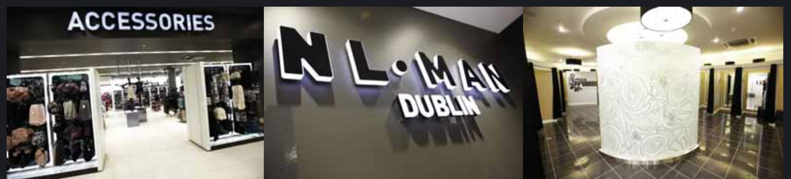
Illuminated crystal-filled acrylic accessories signage | Illuminated wallmounted NL MAN cashdesk signage | Fittingroom screen graphic spot white printed to clear vinyl
